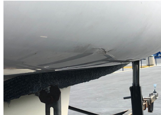
Close up of the damaged Capri. Note the cracking and inverted bottom.
